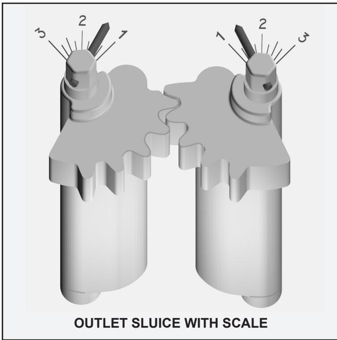
engraved into the top of the stationary insert. Each tablet feeder utilizing one or more riser sections for direct burial will include an adjustable outlet sluice. Follow these steps to adjust the outlet sluice:
