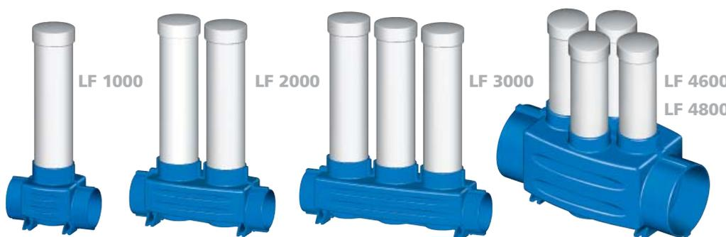
Compact Bio-Dynamic LF Series tablet feeders provide a chemical dose that is ideal for potable water and wastewater systems subject to high organic loading. Manufactured from ABS for durability and easy installation, integral inlet and outlet hubs accept four, six or eight inch piping. LF Series feeders are typically used for residential or small commercial onsite
