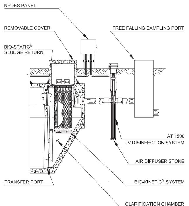
Seamlessly integrating several proven technologies, the Singulair® Direct Bury UV NPDES system's primary treatment platform is the Model 960 equipped with Service Pro® remote monitoring. The UL Listed Service Pro® control center automatically notifies service providers if a component alarm is detected.
