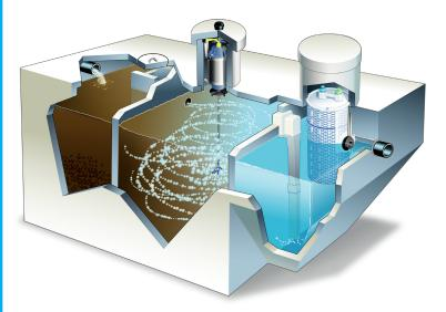
Seamlessly integrating several proven technologies, the Singulair® Direct Bury UV NPDES system's primary treatment platform is the Model TNT equipped with Service Pro® remote monitoring. The UL Listed Service Pro® control center automatically notifies service providers if a component alarm is detected.
