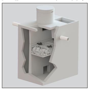
and reduce typical residential flow surges. The flow equalization rate shall be dependent upon the specific loading pattern and the duration of flow surges. At the 600 GPD (gallons per day) NSF Standard 40/245 design loading schedule, minimum performance of the device shall equalize daily flow an average of 50%.
