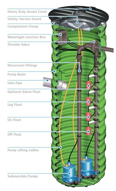
Our Duplex Pump Equipment System provides all the features of our Simplex System, but also gives you the backup protection and extra performance of two pumps. These Duplex Pumping Stations are ideal for greater flows of domestic wastewater and storm water and for pressure sewers, sequential dosing and small municipal collection systems.
