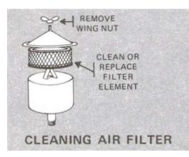
at all times. Check the filter element once a month and clean it as necessary.
