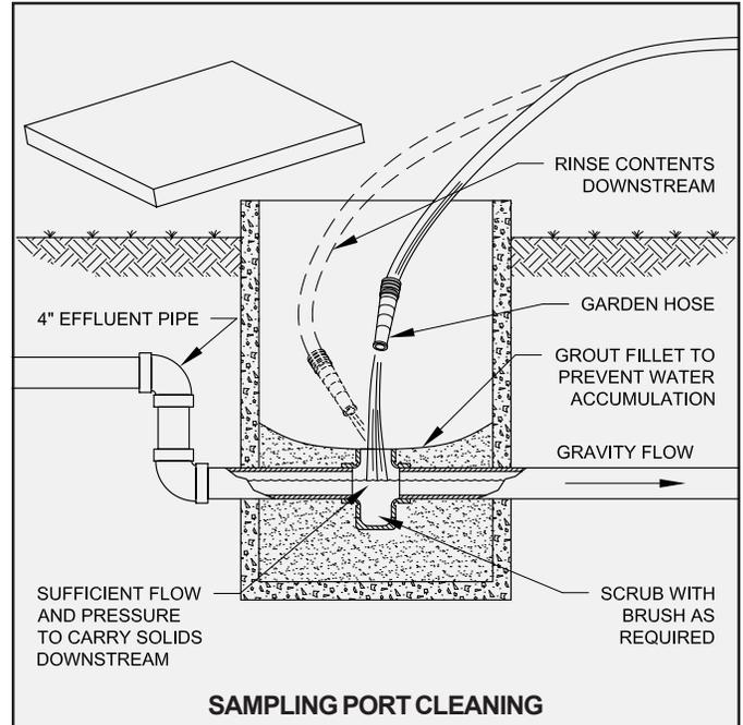
Usually a mild "pressure wash" with a garden hose or similar device will dislodge this growth. Since these solids can be withdrawn by the suction of the sampling pump, this type of maintenance procedure must be performed daily, or more frequently if needed to minimize the growth of biological solids. However, sufficient fall must be designed into the port to prohibit the back up of water into the treatment plant during sampling port maintenance.
