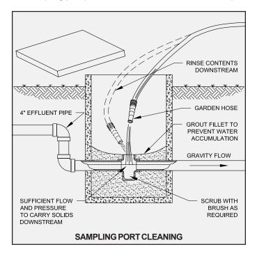
Usually a mild "pressure wash" with a garden hose or similar device will dislodge this growth. Since these solids can be withdrawn by the suction of the sampling pump, this type of maintenance procedure must be performed daily, or more frequently if needed to minimize the growth of biological solids. However, sufficient fall must be designed into the port to prohibit the back up of water into the treatment plant during sampling port maintenance.
