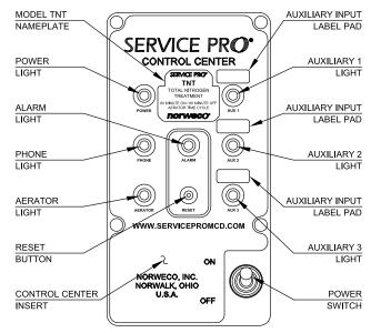
condition to the Service Pro monitoring center. In the event that any of the auxiliary inputs detect abnormal operation of the treatment system auxiliary equipment, the audible and visual alarms shall immediately activate and the telemetry system shall report the alarm condition to the monitoring center. The service provider shall automatically be notified by the Service Pro monitoring center of the specific alarm condition using phone, fax or email.
