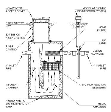
If plastic risers and/or covers are utilized, they must be approved for your application and secured as instructed by the manufacturer. Refer to state and local regulations for applicable codes that may apply to your installation.
