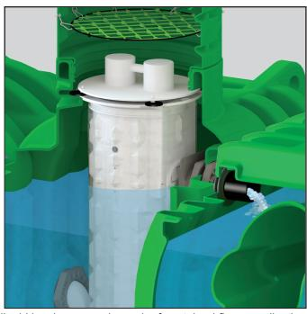
flow dissipates. If the intermittent flow continues to increase, the liquid level may reach a pair of sustained flow equalization ports. With four ports in use, flow through the system increases while continuing to provide flow equalization to all upstream and downstream processes. Peak flow equalization ports are supplied but should not be required in a properly sized system.
