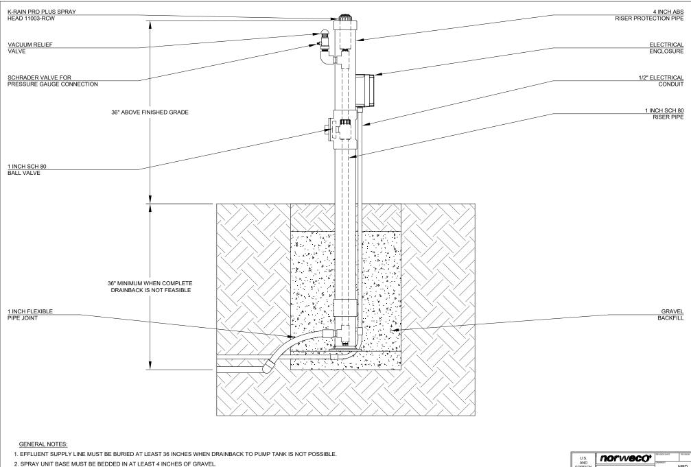
3. SPRAY UNIT MUST BE BACKFILLED WITH GRAVEL TO WITHIN 6 INCHES OF GRADE.
