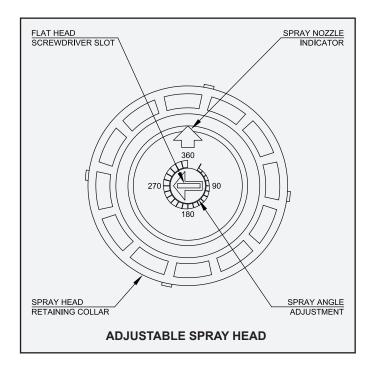
20. The spray heads come with the nozzle number '3' preinstalled at the factory. Nozzles '1', '4' and '6' (also included) can be installed simply by removing the nozzle '3' and installing another. The pressure (pounds per square inch), radius (feet) and flow (gallons per minute) of each nozzle is outlined in the below chart:
